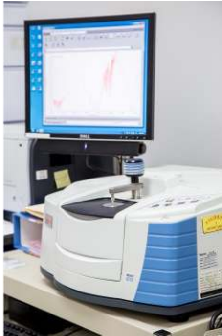
FTIR system (Fourier Transform Infrared Spectroscopy) used to determine detailed chemical composition of test samples Credit: Trelleborg
